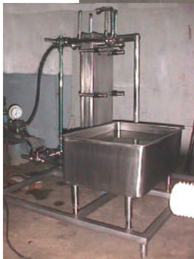
Plate Chiller Unit with Pump & Milk Dump Tank Under Test on Factory Shop Floor
