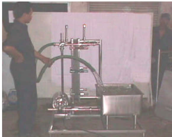
Actual Picture of 1,500 Litres Ice Bank Tank Type Milk Bulk Cooler Under Test on Factory Shop Floor.
