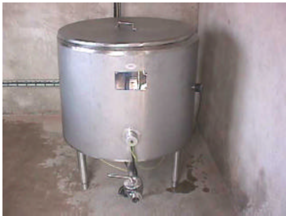
Cleaning In Place (CIP) Unit
