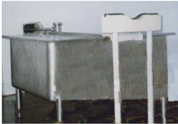
Dump Tank with Can Tipping Bar.
