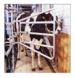
The Encon sequential bailing system is the ultimate means of individual cow control in the milking parlour. All cow spaces are occupied in sequence as cows enter the parlour. Each cow has her own allocated position, which means enhanced cow comfort irrespective of cow size. Sequential bailing offers several advantages and unique features:
